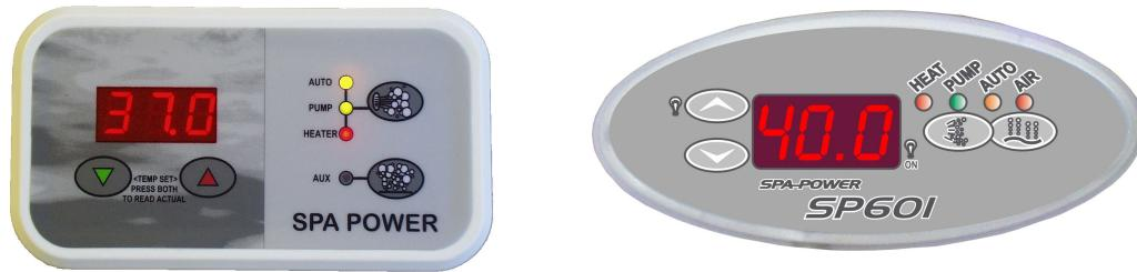
The water resistant poolside control panel features a moulded or webbed waterproof membrane and a polycarbonate overlay that is resistant to pool chemicals. It contains an alarm beeper, soft touch keys and a three digit LED temperature display. All user controls are on this panel except sleep time adjustments, which can be done using the optional sleep control clock that may be fitted to the control box itself.
