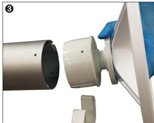
3. Remove the end boss unit from the reel tube, pulling firmly out.
