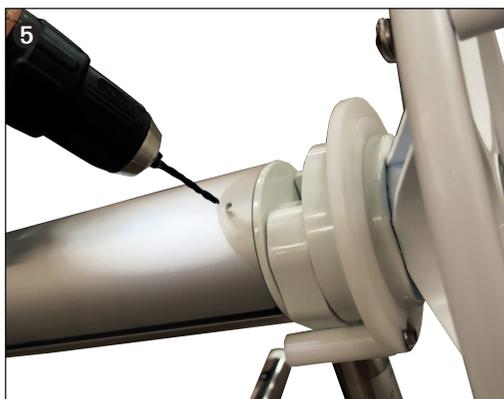
5. Using the existing holes in the reel tube as a guide, drill through into the reduction gearbox end boss using the supplied drill bit.
