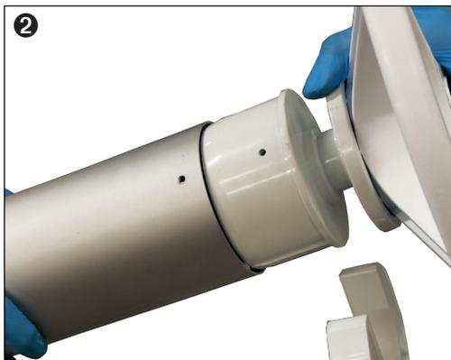
2. Lift the end boss up out of slidlock endstand Y piece.
