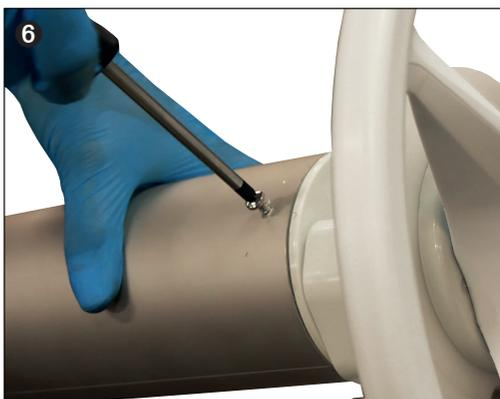
6. Secure the gearbox end boss to the reel tube through the drilled holes using the two supplied screws with a cross/ pozi head screwdriver.
