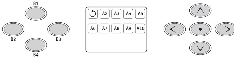
**Note:** Button B2 is ALWAYS unused on TP800 when used with this system. A custom overlay will be required.
