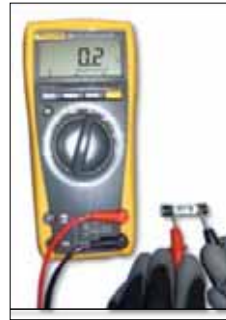
A FUSE WITH THE METER READING "GOOD"
