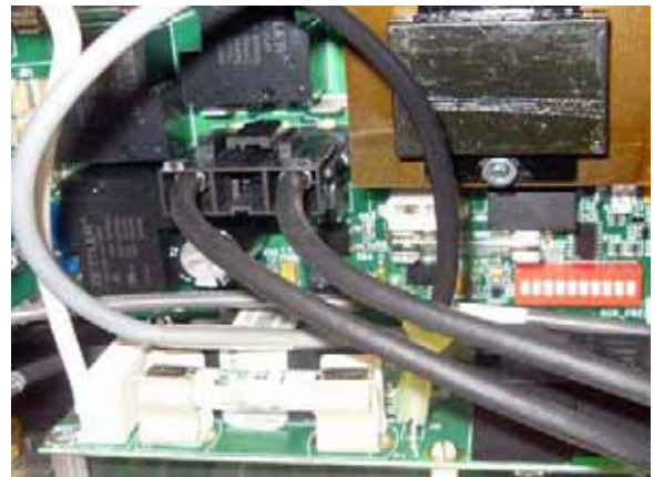
Heater Connector on BP2000/BP2100 Series
