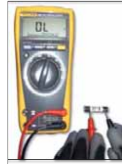
A FUSE WITH THE METER READING "BAD"
