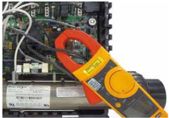
WHEN TESTING AMPERAGE
