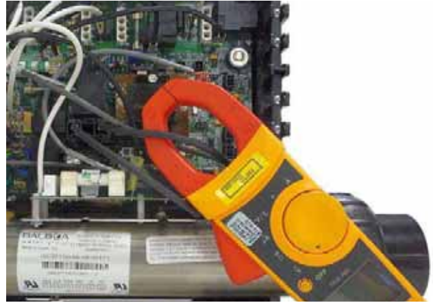
AMPERAGE HEATER TEST BP2100G1
